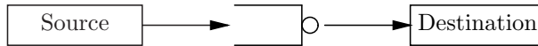
Figure 6.11: The simplest possible topology. A single data flow, with a single intermediate bottleneck router.
